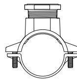
S70 BRASS SADDLE WITH AWWA TAP FOR STANDARD PVC PIPE, ASSEMBLED WATERTIGHT
