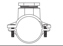
S71 BRASS SADDLE WITH 1-1/2" IRON PIPE TAPS FOR STANDARD PVC PIPE,
