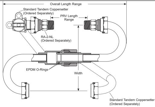
OVERALL **PRV LENGTH** METER SIZE **COPPER TUBE WIDTH** APPROX. **PART** ✓ SUBMITTED LENGTH RANGE RANGE (IN.) O.D. (IN.) (IN.) Wt. Lbs. NUMBER ITEM(S) (IN.) (ln.) 5/8 x 3/4 13/16 12.63-14.63 3.38-5.38 7-1/4 3.2 ST-2-EXP-NL
