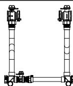
ANGLE BALL VALVE BY ANGLE BALL VALVE (1-1/2" METER)
