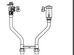
FULL PORT ANGLE BALL VALVE BY CHLORAMINE RESISTANT ANGLE CARTRIDGE DUAL CHECK VALVE (1" METER)
