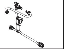
ANGLE BALL VALVE BY ANGLE DUAL CHECK VALVE (5/8" X 3/4" METER)
