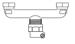
PACK JOINT FOR COPPER OR PLASTIC TUBING (CTS) INLET BY TWO FEMALE IRON PIPE THREAD OUTLETS
