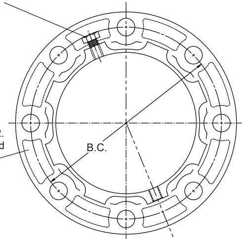
Gasket - NBR (Buna-N) Mechanical Joint Gasket
