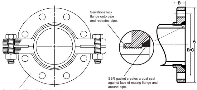
Flange - Ductile Iron ASTM A536 Grade 65-45-12
