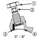
Ductile iron wedges are heat-treated to a hardness of 370 BHN minimum
