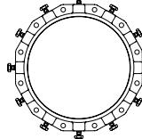
14" - 36" SERIES UFR1500-C MECHANICAL JOINT RESTRAINT FOR C900, C909 OR HDPE PIPE WITH NBR (BUNA-N) GASKET AND 304 STAINLESS STEEL ACCESSORIES
