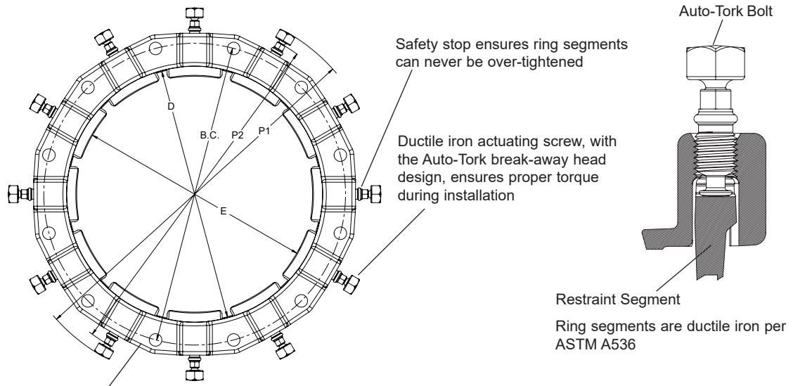
Gland body is of high strength ductile iron per ASTM A536, grade 65-45-12. Compatible with all mechanical joints conforming to ANSI / AWWA C111 / A21.11
