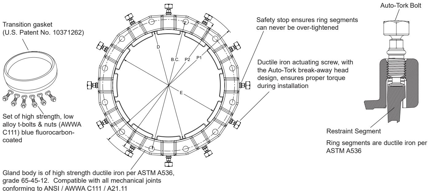
Gland body is of high strength ductile iron per ASTM A536, grade 65-45-12. Compatible with all mechanical joints conforming to ANSI / AWWA C111 / A21.11
