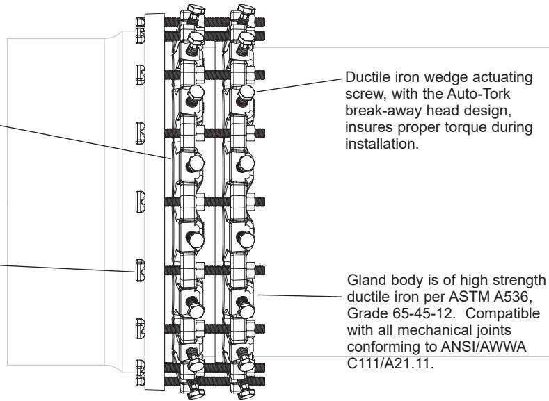
Ductile iron wedge actuating screw, with the Auto-Tork break-away head design, insures proper torque during installation.
