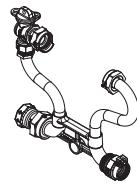
ANGLE BALL VALVE BY METER NUT (5/8" X 3/4" METER)
