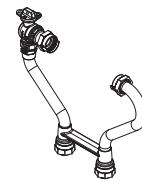
FULL PORT ANGLE BALL VALVE BY METER NUT (1" METER)
