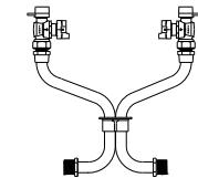
ANGLE BALL VALVE BY \*ANGLE BALL VALVE (5/8" X 3/4" METER)
