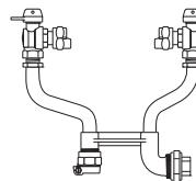
FULL PORT ANGLE BALL VALVE BY FULL PORT ANGLE BALL VALVE (1" METER)
