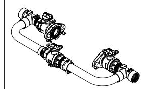
FLANGED ANGLE BALL VALVE BY FLANGED ANGLE BALL VALVE WITH BYPASS (1-1/2" METER)
