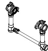
FLANGED ANGLE BALL VALVE BY FLANGED ANGLE BALL VALVE (2" METER)
