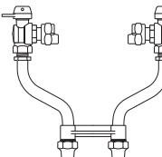
ANGLE BALL VALVE BY \*ANGLE BALL VALVE (5/8" x 3/4" METER)
