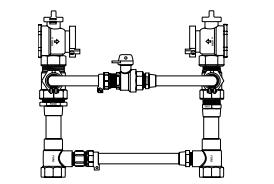
FLANGED ANGLE BALL VALVE BY FLANGED ANGLE BALL VALVE WITH HIGH BY-PASS (1-1/2" METER)
