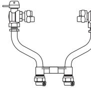
ANGLE BALL VALVE BY ANGLE CHECK VALVE (5/8" x 3/4" METER)
