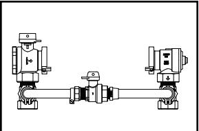
FLANGED ANGLE BALL VALVE BY FLANGED ANGLE CHECK VALVE WITH HIGH BY-PASS (2" METER)
