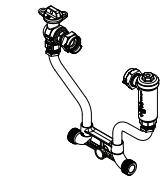
FULL PORT ANGLE BALL VALVE BY ANGLE CARTRIDGE DUAL CHECK VALVE (5/8" X 3/4" METER)
