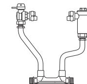
ANGLE BALL VALVE BY ANGLE CARTRIDGE DUAL CHECK VALVE (3/4" METER)
