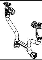
ANGLE BALL VALVE BY ANGLE CARTRIDGE DUAL CHECK VALVE (1" METER)
