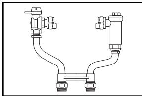
ANGLE BALL VALVE BY ANGLE CARTRIDGE DUAL CHECK VALVE (5/8" x 3/4" METER)
