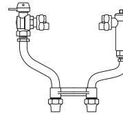
ANGLE BALL VALVE BY ANGLE CARTRIDGE DUAL CHECK VALVE (1" METER)
