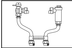
ANGLE BALL VALVE BY ANGLE CARTRIDGE DUAL CHECK VALVE (1" METER)
