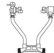
FULL PORT ANGLE BALL VALVE BY ANGLE DUAL CHECK VALVE (3/4" METER)
