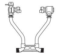
ANGLE BALL VALVE BY ANGLE DUAL CHECK VALVE (3/4" METER)
