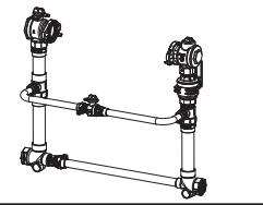
ANGLE BALL VALVE BY ANGLE DUAL CHECK VALVE WITH TEST PLUG (2" METER)
