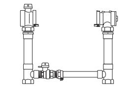
FLANGED ANGLE BALL VALVE BY FLANGED ANGLE DUAL CHECK VALVE WITH BY-PASS (1-1/2" METER)
