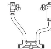
ANGLE KEY VALVE BY ANGLE CARTRIDGE DUAL CHECK VALVE (1" METER)
