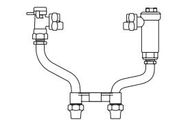
ANGLE KEY VALVE BY ANGLE CARTRIDGE DUAL CHECK VALVE (5/8" x 3/4" METER)
