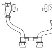
ANGLE KEY VALVE BY ANGLE CARTRIDGE DUAL CHECK VALVE (5/8" x 3/4" METER)
