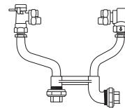
ANGLE KEY VALVE BY ANGLE DUAL CHECK VALVE (5/8" x 3/4" METER)
