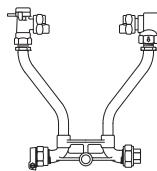
ANGLE KEY VALVE BY ANGLE DUAL CHECK VALVE (5/8" X 3/4" METER)
