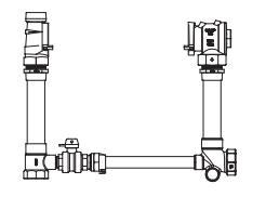
ANGLE KEY VALVE BY ANGLE DUAL CHECK VALVE (2" METER)
