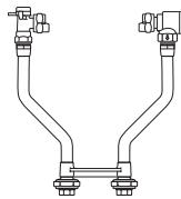
ANGLE KEY VALVE BY ANGLE DUAL CHECK VALVE (3/4" METER)
