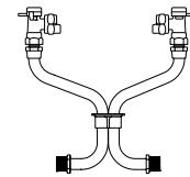
ANGLE KEY VALVE BY ANGLE KEY VALVE (5/8" x 3/4" METER)
