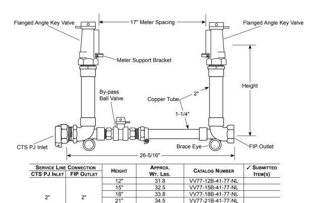
27' Note: Ford recommends using insert stiffeners with plastic pipe or tubing
