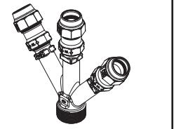
THREE GRIP JOINTS FOR POLYETHYLENE PIPE (SIDR7 PEP) BY SINGLE MALE IRON PIPE THREAD, ASSEMBLED WATERTIGHT
