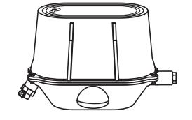
PACK JOINT FOR COPPER OR PLASTIC TUBING (CTS) INLET BY FEMALE IRON PIPE THREAD OUTLET
